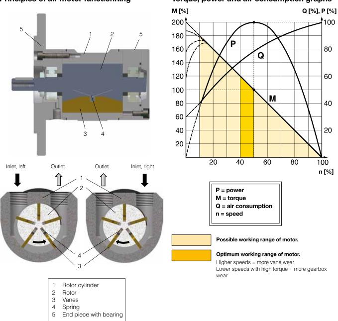
Principles of air motor functionning
