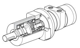
The motor to be used should be selected by starting with the torque needed at a specific spindle speed. In other words, to choose the right motor, you have to know the required speed and torque. Since maximum power is reached at half the motor's free speed, the motor should be chosen so that the point aimed at is as close as possible to the maximum power of the motor.
