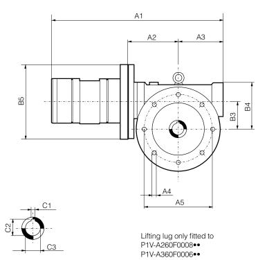
As standard, the motor has a hollow shaft with key slot. Please refer to next page for a dimension sketch of the single ended and double ended shafts.
