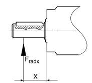
Fig. 4: Force applied at distance X
