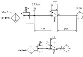
Shut-off, filtering, pressure regulation and control valve
