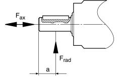
Fig. 1: Loading on output shaft.
