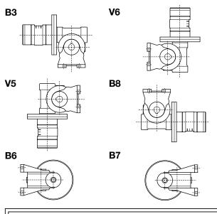
**Note:** Oil-bath gearboxes mean that the installation position must be decided in advance. The installation position determines the volume of oil in the gearbox and location of oil filling and drain plugs.
