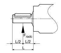
Fig. 3: Force applied at centre of shaft
