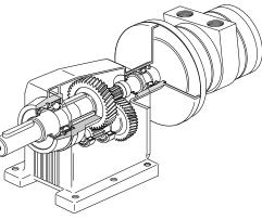
Helical gears are characterised by high efficiency. Several reduction stages permit relatively high gear ratios. Central output shaft and simple installation with flange or foot.
