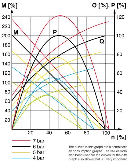
P = powerQ = air consumptionM = torquen = speed
