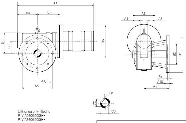
As standard, the motor has a hollow shaft with key slot. Please refer to page 36 for a dimension sketch of the single ended and double ended shafts.
